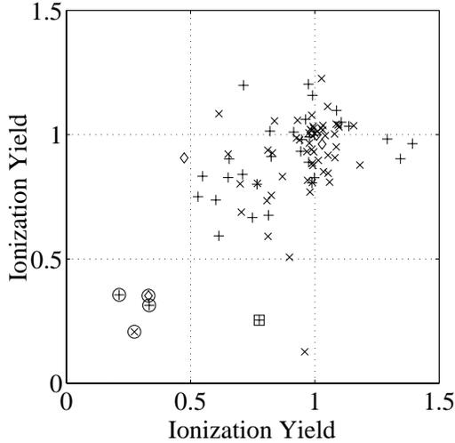
Figure 2. Scatter plot of ionization yields for veto-anticoincident double-scatters in the top and middle (+), top and bottom ( $\diamond$ ), or middle and bottom ( $\times$ ) Ge detectors. Circled (boxed) events are tagged as a nuclear recoil in each (one) detector. Both events with ionization yield  $Y < 0.45$  in only one of the two detectors hit have the low-yield hit in the outer electrode, consistent with expectations for misidentification of electron recoils in the outer electrode.
