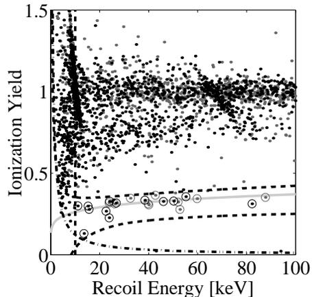
Figure 1. Ionization yield ( $Y$ ) vs. recoil energy for unvetted single scatters in the 3 Ge detectors. Solid curve: expected position of nuclear recoils. Dashed curves: mean nominal 90% nuclear-recoil acceptance region. Dashed line: 10 keV analysis threshold. Dot-dashed curve: mean threshold for separation of ionization signal from amplifier noise. Circled points: nuclear recoils.
