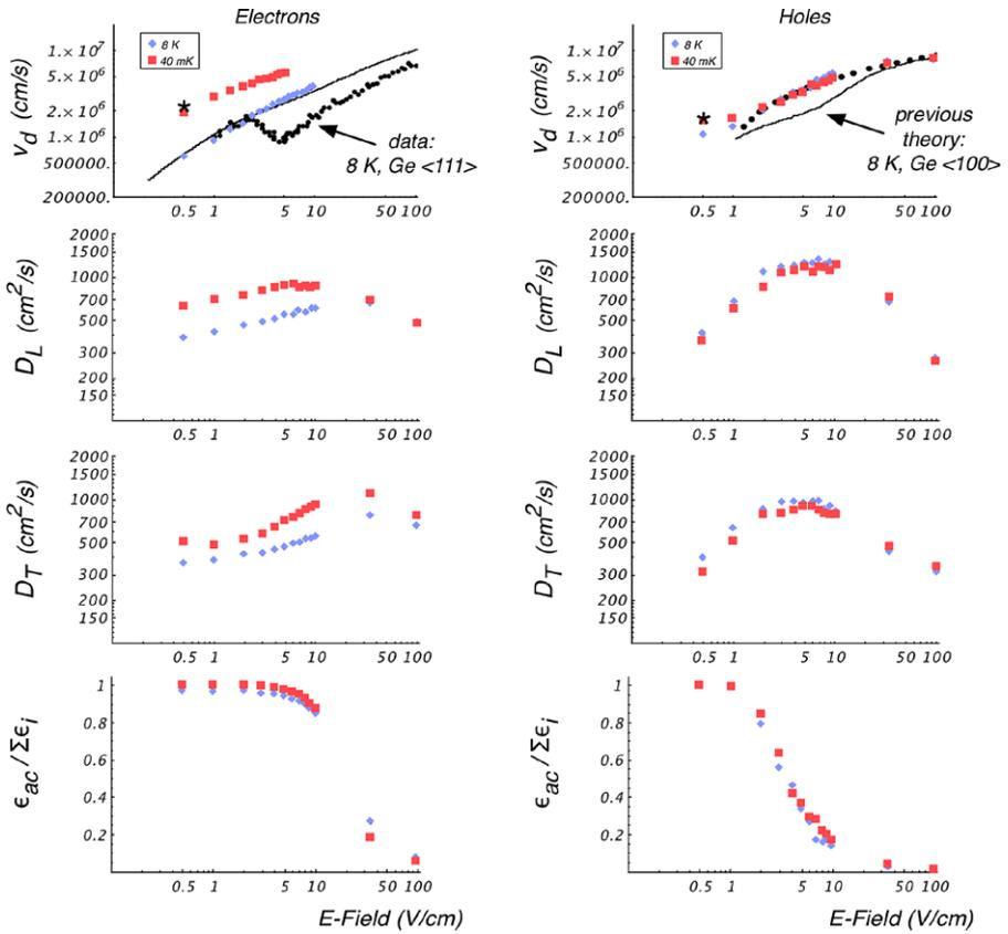
**Fig. 1** (Color online) A comparison of electrons and holes, 8 K (*diamonds*) and 40 mK (*squares*). *Top* graphs show drift velocity compared to pre-existing 8 K theory (*continuous lines*) and experiment (*points*) [1–4]. *Asterisks* (\*) denote data from [8]. The next *two rows* of graphs show simulated diffusion, longitudinal and transverse. The *bottom row* shows the ratio of energy dissipated by acoustic phonon emission to that of all phonon emission processes
