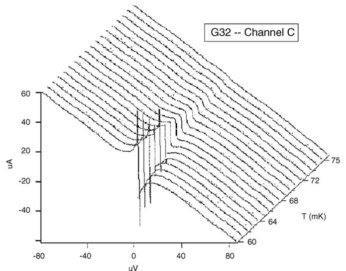
Fig. 2. The temperature variation of  $I$ – $V$  curve for one phonon sensor. The  $x$ -,  $y$ - and  $z$ -axis, respectively, report bias voltage, sensor temperature and the sensor current. With this set of curves we can estimate the  $I_c$  and  $T_c$  of each sensor.
