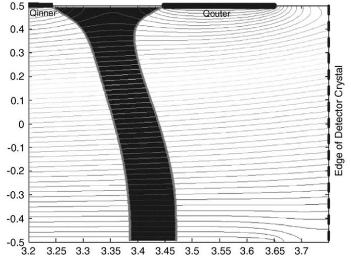
Fig. 2. Electric field lines traced from gap-side edges of  $Q_{\text{inner}}$  and  $Q_{\text{outer}}$  define the boundary of the region we believe causes the funnel. Equipotential lines describe the distorted electric field.
